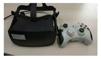
FIGURE 1 The Oculus Rift CV1 and Betop gamepad controller used in the experiment
